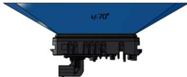
Figure 26: Keep-Out Zone - Azimuth
