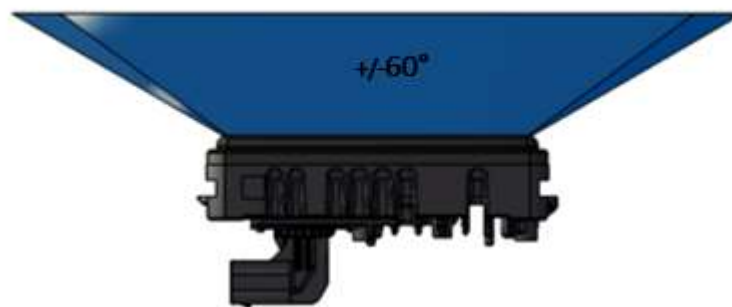
Figure 23: simplified Radiation Cone ARS 548 RDI - Azimuth (without any tolerances)
