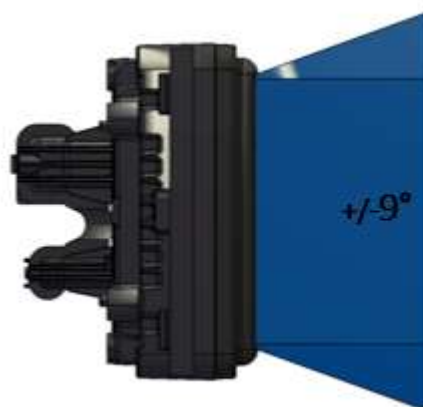
Figure 23: simplified Radiation Cone ARS 548 RDI - Azimuth (without any tolerances)
